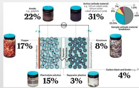
Typical composition of a battery cell. (Argonne National Laboratory)
