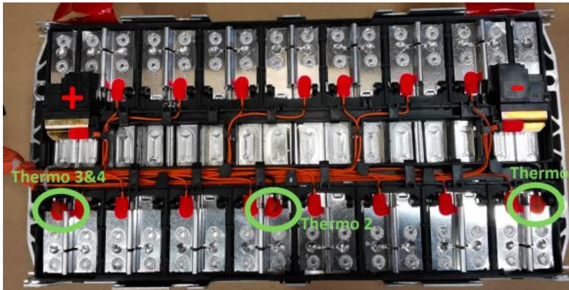
Figure 4. BMW group battery module
